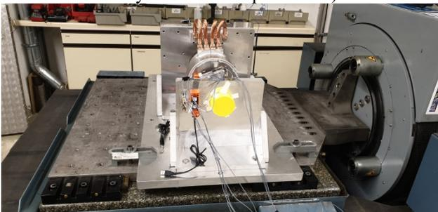
Figure 9: the coupler on the shaking table
