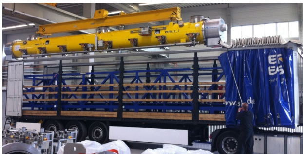
Figure 1: Cryomodule being prepared for transport.
