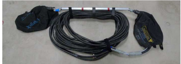
Figure 6: Shielding gas purging tool for the GRP.
